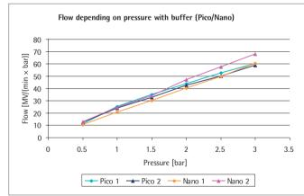
Flow rate >10 MV/(min  $\times$  bar)
