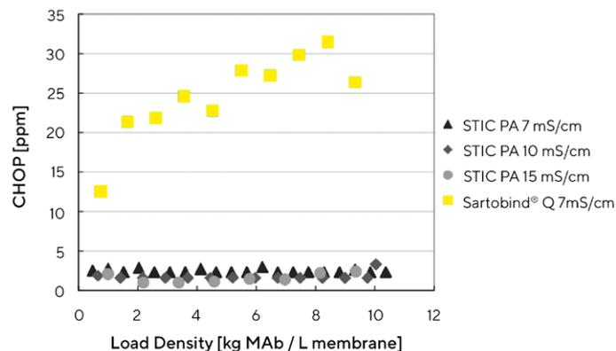
Fig. 1: HCP concentration in Sartobind STIC® PA and Sartobind® Q pools as a function of load density at various conductivities. Sartobind STIC® PA shows higher HCP clearance than Sartobind® Q at conductivities up to 15 mS/cm.
