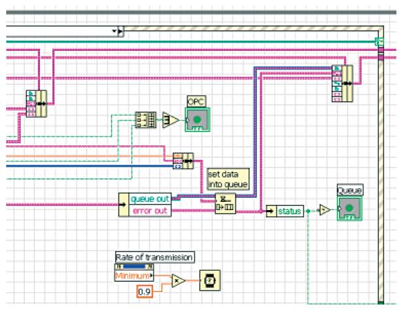
Even the error flags are bundled and displayed in the "OPC" LED. The status of the queue is displayed in the "Queue" LED. In addition, a standby time is activated that is a little less than the set sensor rate ("Rate of transmission" in the Browse to OPC Item page).
