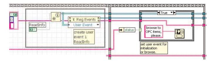
When the server and the device have been found, this triggers a user event that triggers the reading of the device ID in the producer loop.
