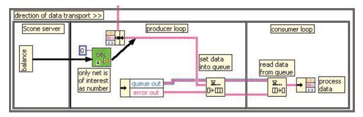
Because of the Panel Close option, the "Exit" key is set to "True" via the corresponding local variable. A signal is sent via "queue" to the consumer loop. This "wakes up" the consumer loop, which reads the local variable "Exit" that now is set to "True": the consumer loop is then closed in this way. Therefore, the "Exit" event of the producer loop waits a short period of time and then transmits "True" to the conditional loop terminal (stop if "True").
