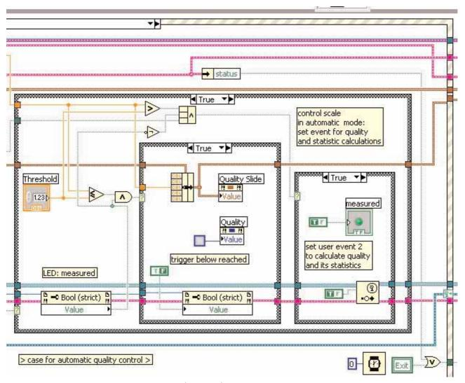
The basic conditions are checked in the "and node" (top center) (Value > threshold and stability, the event is not yet triggered). The last condition comes from the display value of the "measured" LED.
