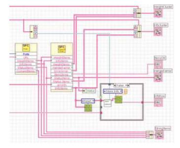
The Infoltems are then used immediately to read the ID information from the connected device.
