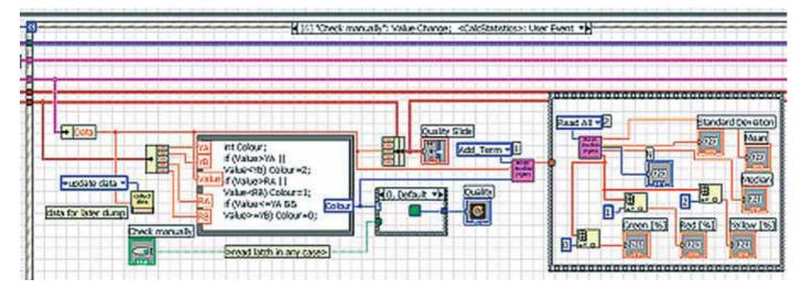
An index for the color to be displayed is calculated here in the formal nodes. This index is entered in the CalcStatistics.vi sub (violet icon) and calculated there using the percentage numbers. In addition, the statistical measurements are calculated, i.e. quantity, mean value, median and standard deviation. The events are read and output in the right sequence structure.
