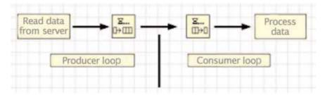
In order to transmit data, it must be set in a queue (queue icon). The consumer loop waits in its "timeout event" for the receipt of new data. During this wait period no CPU time is required. In addition, events in the consumer or producer loops can be executed asynchronously.
