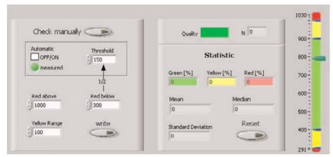
(1) Sets the parameters in the event "Red above," "Red below," "Yellow." A formal node is used to calculate the parameters.
