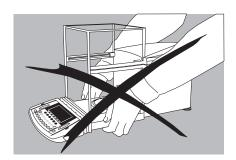
Do not lift the balance by the draft shield or the front panel, as this can result in damage.
