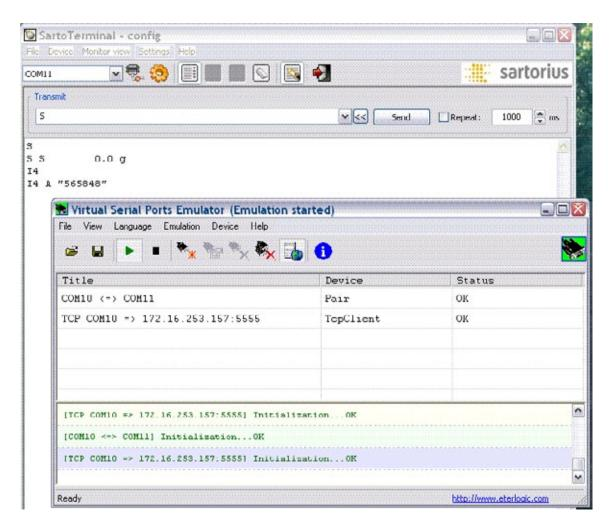
8) Connect SartoTerminal with cubis (Button near "COM 11"). If connection is OK, points RTS, DTR,CTS and DSR will become green (down right) and symbol DISCONNECTED changes to CONNECTED.
