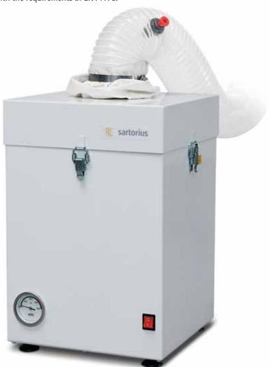
The filter unit with an HEPA H14 filter is freestanding to effectively prevent vibrations. The "bag in, bag out" filter system allows the filter to be changed quickly and contamination-free.
