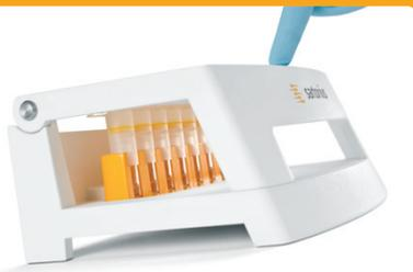
Claristep® Filter units press liquid through each membrane by an air pocket that forms over each filter unit when the station lid is closed. This air pocket is released when you stop holding down the lid – you will feel it in your fingertips!
