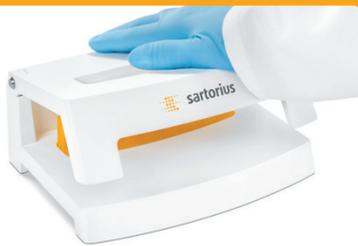
Apply slight uniform pressure with your hand to start sample clarification. You will feel a certain resistance while liquid is pressed through each membrane.
