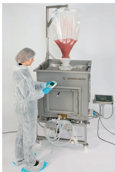
200L Palletank for Magnetic Mixer equipped with the powder transfer bag for the mixing trial
