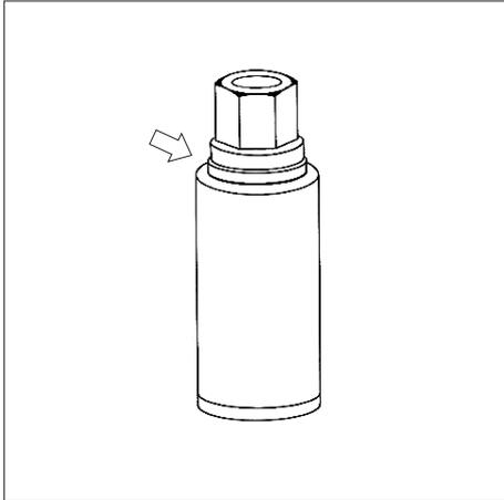
Fig. 23: First notch (steaming position)
