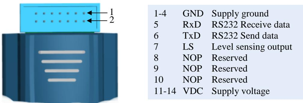
Figure 8. rLine connector pin descriptions
