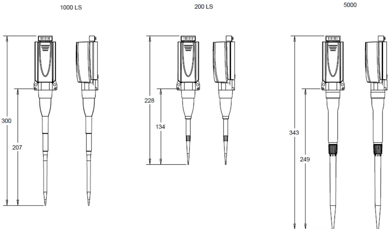
Figure 6. rLine models dimensions with tips
