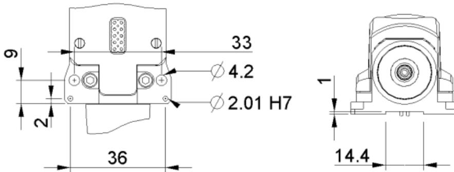
Figure 7. rLine location guide dimensions
