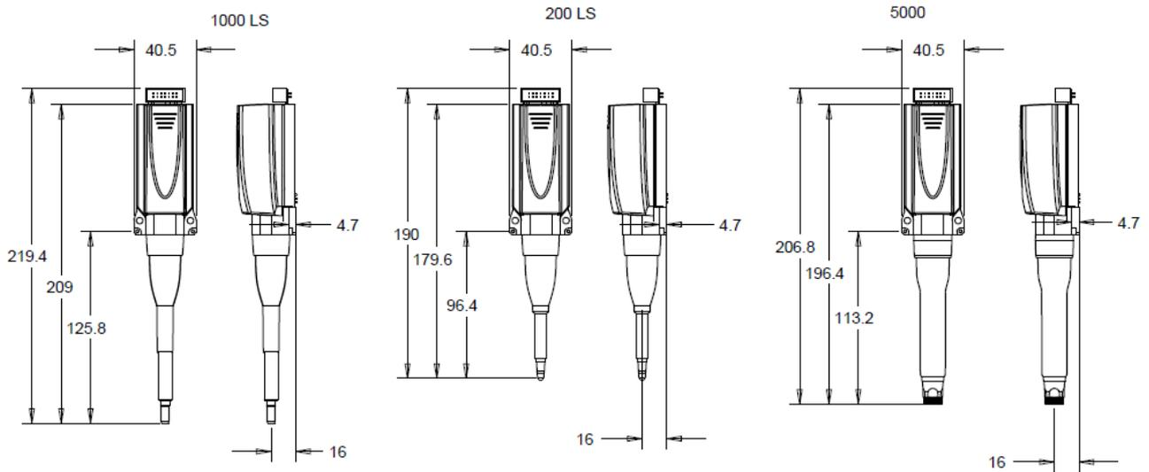
Figure 5. rLine models dimensions without tips
