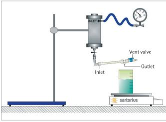
Fig. 2: Experimental set-up of small-scale filtration using Virosart<sup>®</sup> Media lab module 5 cm<sup>2</sup>
