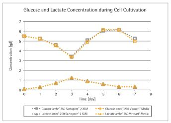
Fig. 9: Glucose and lactate concentration during CHO fed-batch cultivation in an ambr<sup>®</sup> 250 modular bioreactor system using media filtered with a Virosart<sup>®</sup> Media and a standard Sartopore<sup>®</sup> 2 XLM for comparison
