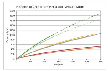
Fig. 4: Filtration of five different cell culture media with Viorsart $^{\circ}$  Media at constant pressure of 2.0 bar | 30 psi for 240 min filtration
