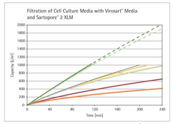
Fig. 6: Filtration of five different cell culture media with Virosart<sup>®</sup> Media and Sartopore<sup>®</sup> 2 XLM as pre-filter at constant pressure of 2.0 bar  $\mid$  30 psi for 240 min filtration
