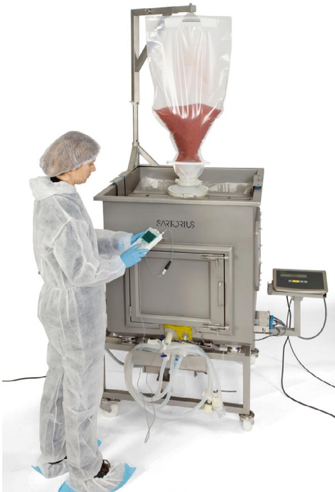
200 L Palletank® for Magnetic Mixer equipped with the Powder Transfer Bag System for the mixing trial
