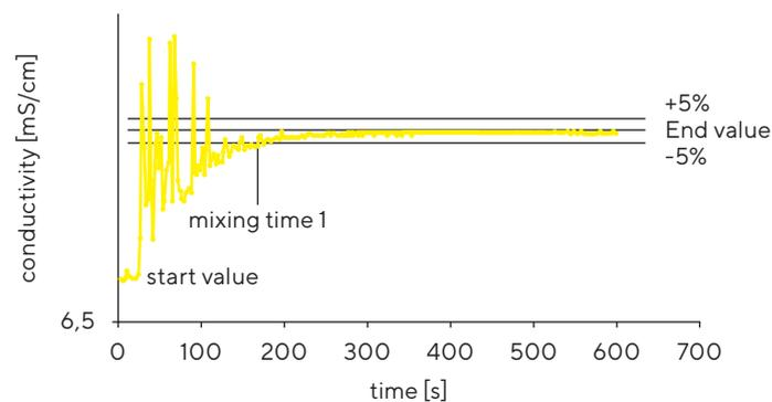
**Figure 1:** General principle of mixing time determination via conductivity
