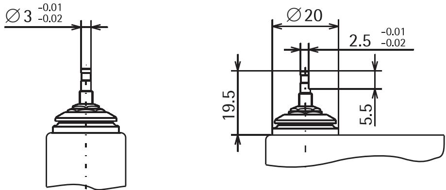
The transducer can be installed on this stud using clamps, for example. The transducer should consist of conductive, non-magnetic material in order to minimize electrostatic and magnetic interference. The transducer must weigh  $5 \text{ g} \pm 0.1 \text{ g}$ , so that the full weighing capacity of 20 g can be achieved. It must be smaller than 10 g in order to use the internal calibration function. Remove the transducer when transporting the weigh cell.
