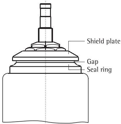
The cell has a rating of IP44 in normal weighing mode. This protection rating is only valid when there is a gap between the shield plate and the seal ring.
