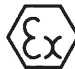
2 **Equipment or Protective systems intended for use in Potentially Explosive Atmospheres - Directive 2014/34/EU**
