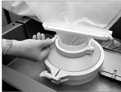
Figure 1: Docking of the 15 L Powder Bag onto the Flexel® Bag for Magnetic Mixer
