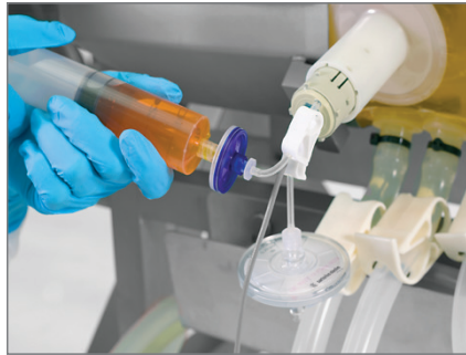
Figure 3: Calibration of the single-use pH probe
