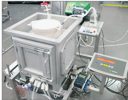
Figure 4: 50 L Flexel® Bag for LevMixer® in 50 L Palletank for LevMixer® (weighing)
