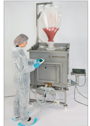
200 L Palletank for Magnetic Mixer equipped with the Powder Transfer Bag System for the mixing trial
