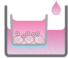
Add 200 µL of chemoattractant or controls to reservoir plate. Place the insert into the pre-filled reservoir plate and image in Incucyte® Live-Cell Analysis System.
