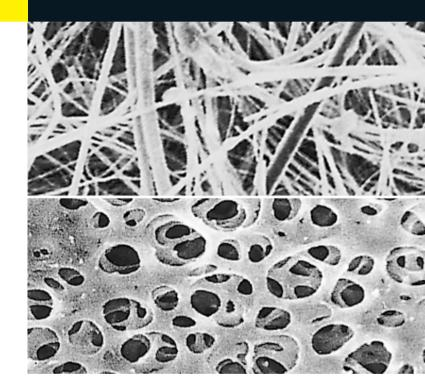
Sartoclean® GF filter cartridges combine absolute retention performance by membrane filtration with high adsorptive power by glass fiber fleeces. Therefore Sartoclean® GF are ideally suited for removal of colloids and lipids as well as defined particle retention and bioburden reduction for a broad range of bio-pharmaceutical applications.
