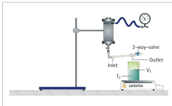
Figure 1: Experimental set-up for spiking study using Virosart® Media lab module 5 cm<sup>2</sup>
