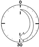
After connection to AC power and before each calibration/adjustment, allow the scale to warm up for approx. 30 min.
