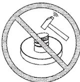
Never use a hammer to close the lid of a paint can while it is still on the weighing pan.
