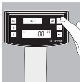
2. Press the **F** formulation key (7) several times to select the conversion factor “0.25” used in this example.
