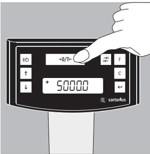
Hold down the  $\rightarrow 0/T \leftarrow$  key (5) for 2 sec. When 5000 is displayed, release the key.
