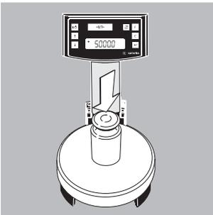
Center the calibration weight on the weighing pan (11). Calibration/adjustment is performed automatically. After calibration and adjustment, remove the weight.
