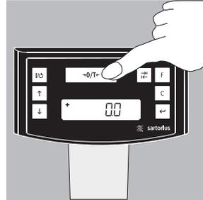
If a different readout is displayed, zero or tare the scale using the
