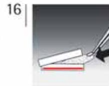
Place the filter on the Nutrient Pad, avoid to entrap air bubbles under the filter.
