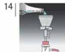
Open the valve and filter the sample. Rinse with a few mls of sterile water to remove all product residues or inhibitors that might be contained in the sample. Close the valve again.
