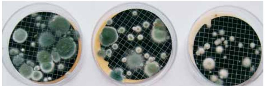
It generally proves practical to place petri dishes with agar or with moistened nutrient pads plus a membrane filter, directly in the filling room and to leave them exposed there for several hours – for instance during a filling shift. This offers a direct correlation to the bacterial load that the filling heads are exposed to. As can be clearly seen from the adjacent images, the bacterial load can vary greatly.
