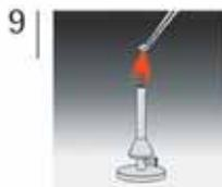
The forceps should always be stored in a small glass with alcohol. Take it out of it and flame it. Let it cool off for a few seconds before use.
