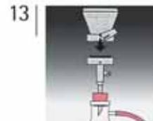
Place the funnel on the filter support and close it with the clamp.
