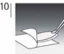
Open the cover of the sterile single-packed filter without touching the filter with your fingers. Take it out together with the yellow protective disc with the sterilized forceps.
