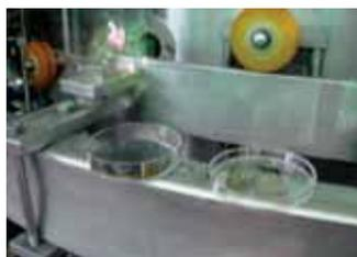
This method can also be carried out by vertically attaching petri dishes with culture medium in the production facilities (mainly to the filling block, the filter, the labeling machine etc.) and leaving them there for approximately 2 hours before removing them and incubating them for 2 to 3 days.
