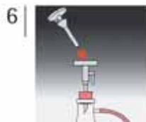
Open the vacuum valve and carefully flame the filter support for ~10 sec. Close the vacuum valve again.
