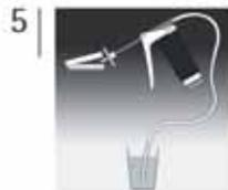
Wet the pads with 3,5 ml of sterile, deionized or distilled water.
