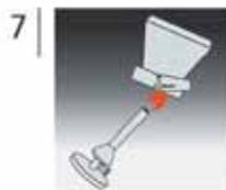
Take the funnel at both sides of the clamp and flame it from its lower side. Then place it on the filter support.
