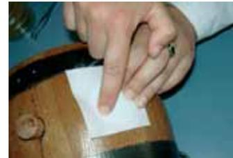
This method is used to test the bacterial contamination of relatively smooth surfaces.
