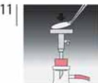
Place both together on the filter support. The yellow protective disc will coil up by the water residues of the frit.
