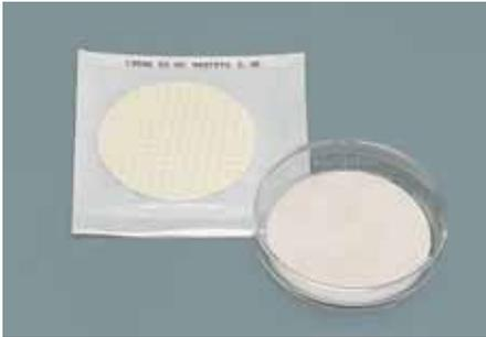
Nutrient pad set with membrane filter
