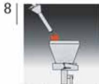
Open the vacuum valve again and flame the inside of the funnel.
