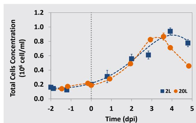
**Figure 4.** Vero cells growth before and after infection by PPRV for the 2L (blue) and 20L (orange) STB. Dashed gray line: time of infection. DPI: days post-infection. Error bars represent: (i) for the 2L STB - standard deviation of two independent cultures, (ii) for the 20L STB - standard deviation of 4 independent cell counts.
