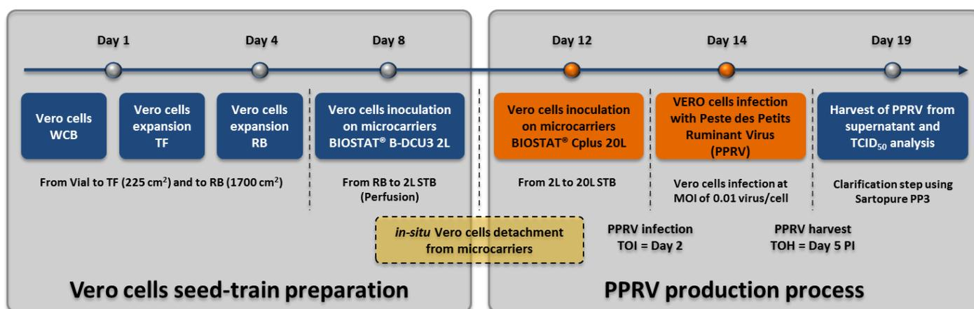
**Figure 2.** Vero cells seed-train preparation and PPRV production process in the BIOSTAT® Cplus 20L STB. Abbreviations: MOI – Multiplicity of infection; RB – Roller bottle; TF – Tissue culture flask; TOH – Time of harvest; TOI – Time of infection; WCB – Working cell bank
