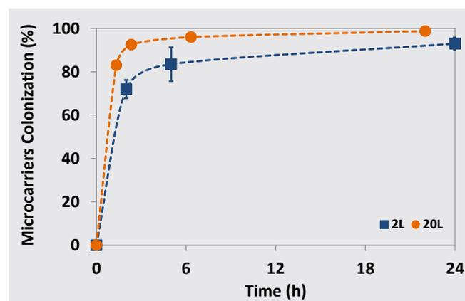
**Figure 3.** Kinetics of MC colonization for the 2L (blue) and 20L (orange) STB. Error bars represent standard deviation of 3 independent measurements.
