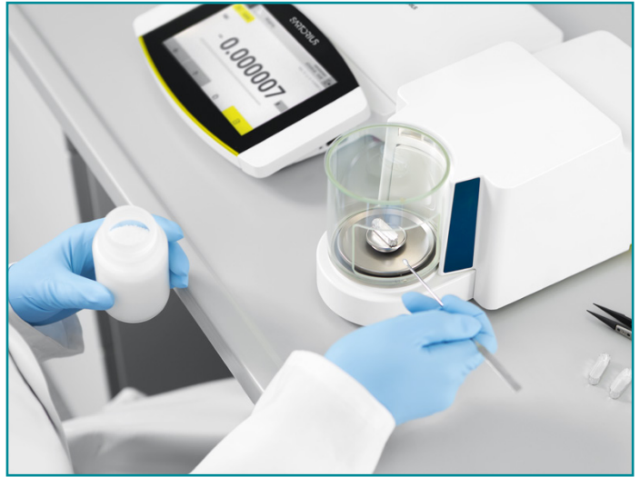
Figure 5. The proximity sensors are located on the left and right of the glass draft shield. The sensors detect the operator's hand and automatically open the draft shield, and close it when the hand is moved out of the sensor's detection range.
