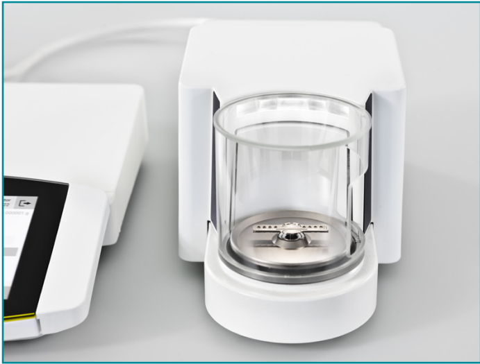
Figure 4. Microbalance weighing module with crystal clear glass draft shield and sample holder for stent weighing. The draft shield base plate and sample holder are made of titanium. The round, flat weighing pans with a diameter of 20/30 mm and 50 mm, which are part of the standard delivery contents, are also made of high-quality, non-magnetic titanium. The weighing chamber can be disassembled easily and within a few seconds for cleaning purposes.
