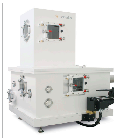
Figure 2: Mass comparator Sartorius CCL1007.
