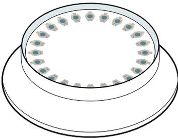
Make sure to position the tubes with the back side toward the outside of the rotor in order to form the pellet on the back wall of the tube.
