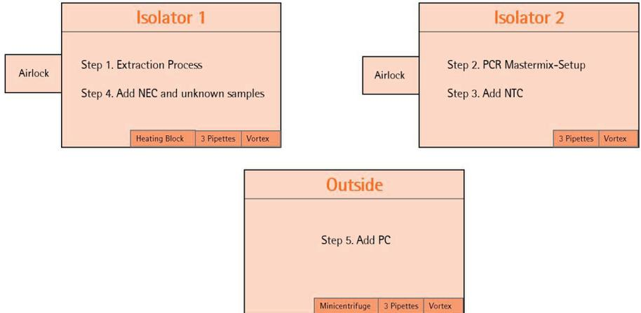
It is also possible to connect Isolator 1 and Isolator 2 via an airlock so that you can transfer your PCR-tubes after Step 3 directly from Isolator 2 into Isolator 1. Please note that you need an additional airlock for Isolator 2 in this case.
