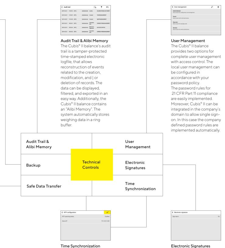
The Cubis<sup>®</sup> II balance supports automatic time synchronization via Network Time Protocol (NTP). An accurate time stamp is elemental for trustable records.
