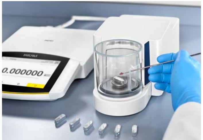
Figure 1: Weighing smallest amounts of substances on a microbalance.
