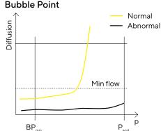
If the measured flow is below the min when "P<sub>end</sub>" is reached, the test is considered as failed and an explicit error message is displayed, and optionally, printed.
