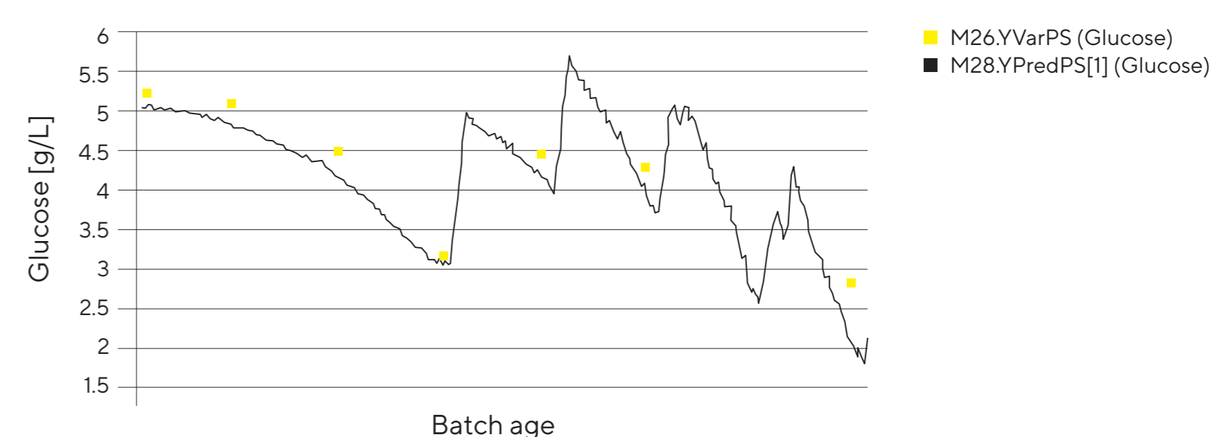
Figure 7: Graph Showing the Prediction of the Raman Glucose Model Built in Ambr ® of the Glucose Concentration in the Biostat STR ® 200.
