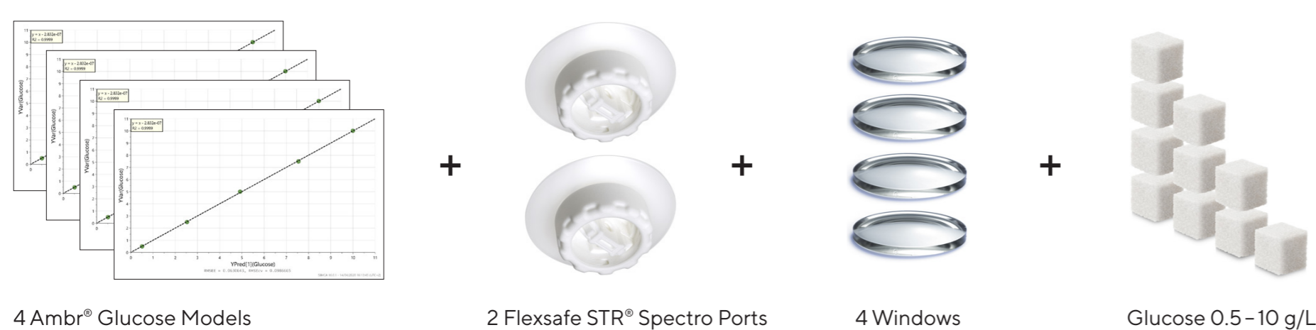
Figure 4: Schematic of the Experimental Setup: The 4 Different Ambr ® Glucose Models From Above Were Applied to Predict the Glucose Concentration Of 4 Different SU Port/Window Combinations.
