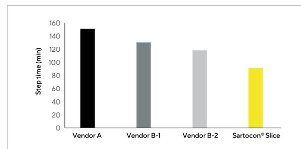
Hydrosart® processing time was significantly faster compared to the other crossflow membranes used in this study.
