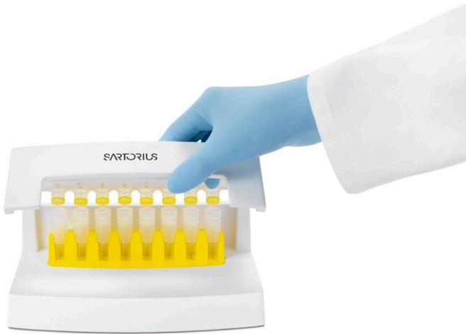
2. Apply slight uniform pressure with your hand to start sample clarification. You will feel a certain resistance while liquid is pressed through each membrane.
