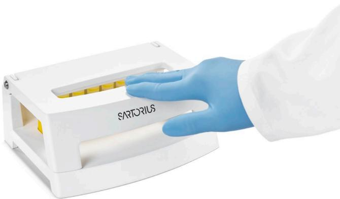
4. Claristep® Filter units press liquid through each membrane by an air pocket that forms over each filter unit when the station lid is closed. This air pocket is released when you stop holding down the lid—you will feel it in your fingertips!
