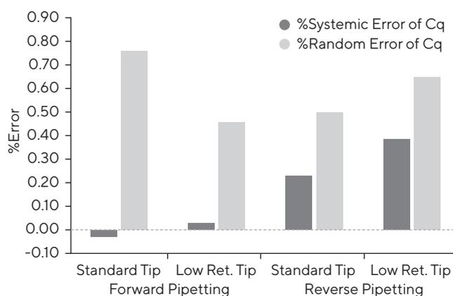
Figure 2: %Error of Cq (cycle of quantification) for forward and reverse pipetting of Master mix. %Systemic error of Cq (cycle of quantification) and %Random of Cq are shown. For each data point, n = 8. Forward pipetting gives a low systemic error compared to reverse pipetting (gray bars). Standard Tip—Sartorius Safetyspace Filter Tips, Low Ret. Tip—Sartorius Safetyspace Low Retention Tips.
