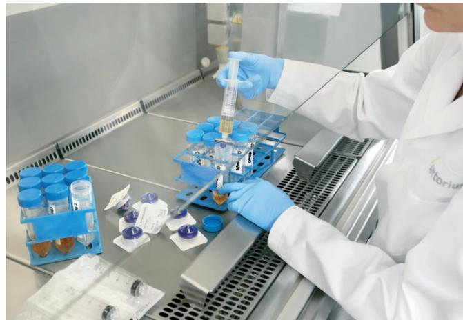
Figure 1: Initial clarification and subsequent sterile filtration of cell culture supernatants under aseptic conditions using a Minisart® High Flow syringe filter with a pore size of 0.22  $\mu\text{m}$ .
