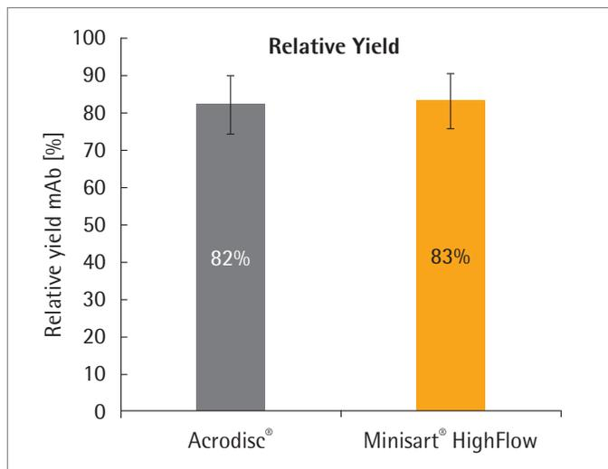
Figure 4: Average values of the relative yield [%] of various mAb products. The relative yield of a sample is the ratio of the total mAb quantity in the filtrate to that in the unharvested cell culture. As a result, we found no difference between both filter types regardless of the syringe filter design and the number of filters used.
