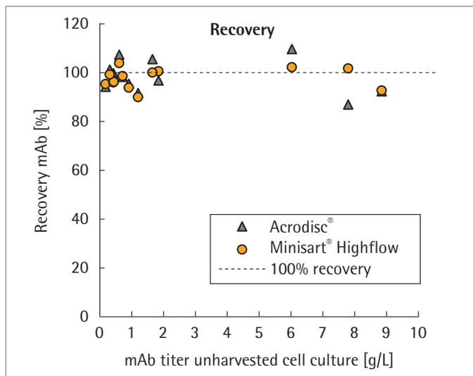
Figure 3: Recovery [%] of mAb products in relation to the mAb titer of the unclarified cell culture; this recovery was not affected by the syringe filter type and was, on average, 98.2% for Acrodisc® and 97.7% for Minisart® High Flow. No impact of the syringe filter used was observed on mAb recovery in a range of 0.3 g/L to 8.8 g/L of the cell culture titers.
