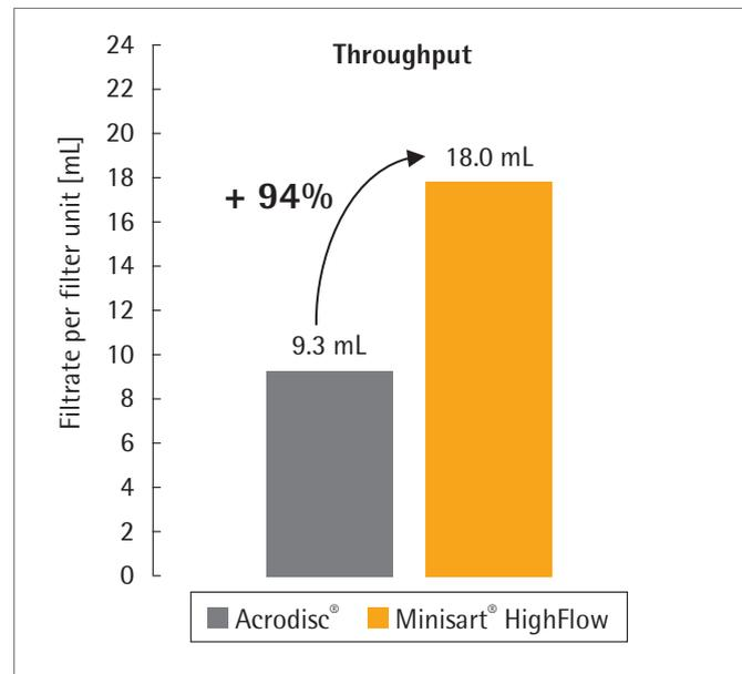
Figure 5: CHO cell culture supernatants were filtered through two different syringe filter types (0.22 µm): Sartorius Minisart® High Flow and Pall Acrodisc®. The average throughput per syringe filter was determined. Differences in throughput between both filter types were probably not caused by the difference in effective filtration area (Acrodisc®: 5.8 cm<sup>2</sup>, Minisart® High Flow: 6.2 cm<sup>2</sup>), but most likely by differences in structural membrane design.
