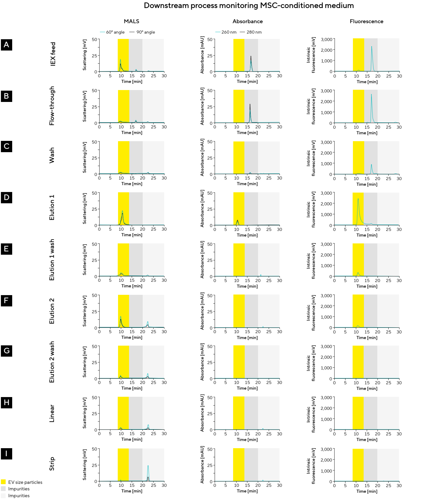
Figure 10: AEX step evaluation using multi-detector analytical chromatography. SEC with inline MALS, UV absorbance, and intrinsic fluorescence detection was used to evaluate the distribution of particles and impurities: (A) load, (B) flow-through and (C) wash samples. Comparison of eluates: (D and E) Elution 1 and wash, (F and G) Elution 2 and wash, as well as (H) linear (in which salt concentration was increased from 400 to 1,000 mM) and (I) strip (in which salt concentration was kept as 1,000 mM). n = 3 independent downstream runs.
