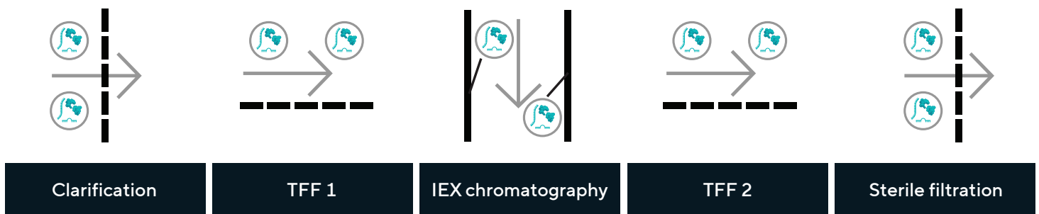
Figure 1: Downstream purification process for MSC-derived EVs
