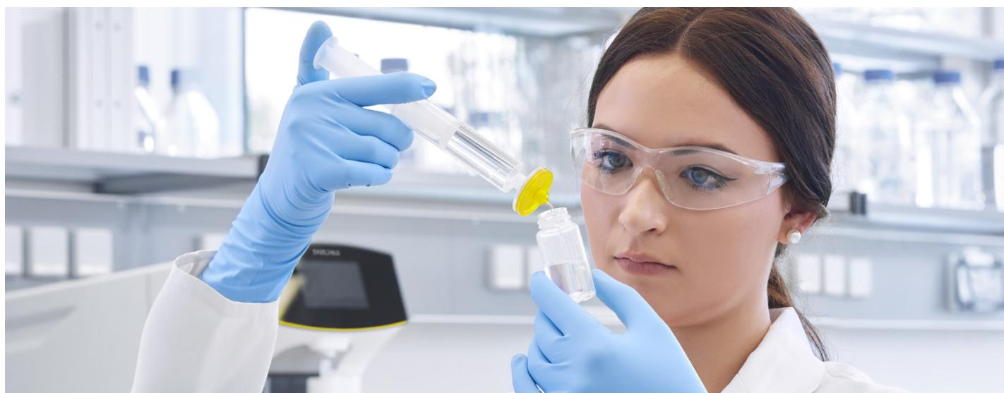
Figure 4: Filtration of a water sample using the syringe filter Minisart® High Flow with pore size of 0.45 µm (yellow housing).
