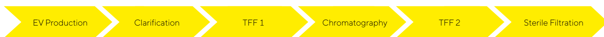
Figure 1: Schematic Process Flow Representing Unit Operations Involved in the EV Purification Process
