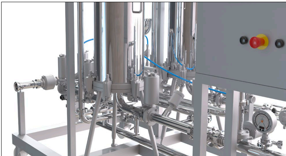
Figure 3: Detail of the Duo Jumbo Star System
