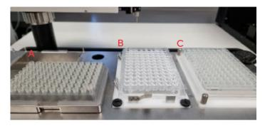
**Figure 1:** Cooled destination deck tray. (A) Rack containing 500  $\mu$ m plastic PrecisionTips; (B) 96 well destination tray for organoid transfer; and (C) Cooled PCR plate containing 30  $\mu$ l Matrigel in each well at approximately 0°C.
