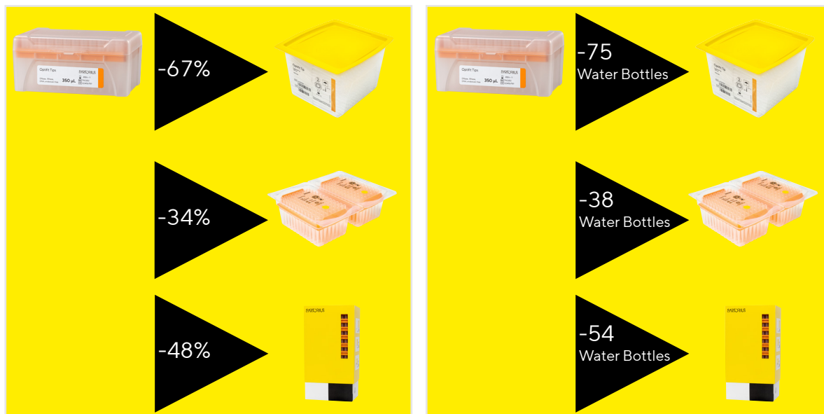
Figure 2. Reduced weight of total plastic material per 960 tips when compared to single tray package. Comparison performed using 350 µl Optifit Tip products.
