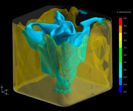
**Figure 5:** Simulation of Vertical Velocity in the Flexsafe® Pro Mixer (3D View)
