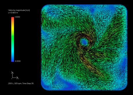
Figure 4: Top View of Vortex Formation in a Flexsafe<sup>®</sup> Pro Mixer
