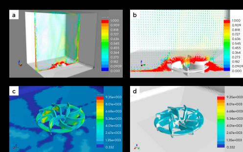
**Figure 6:** CFD Data for 200 L Flexsafe<sup>®</sup> *Pro Mixer at 450 rpm.*
