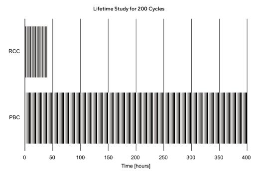
**Figure 5:** Comparing the Time to Complete a Lifetime Study for RCC and PBC. RCC Cycle Time Is 12 Minutes and PBC Cycle Time Is 2 Hours in This Example.
