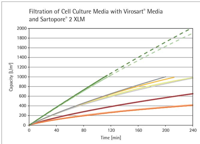
Fig. 6: Filtration of five different cell culture media with Virosart® Media and Sartopore® 2 XLM as pre-filter at constant pressure of 2.0 bar | 30 psi for 240 min filtration
