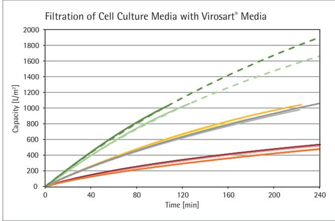
Fig. 4: Filtration of five different cell culture media with Virosart® Media at constant pressure of 2.0 bar | 30 psi for 240 min filtration
