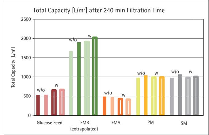
Fig. 6: Total capacity after 240 min filtration time at constant pressure of 2 bar | 30 psi in duplicate runs with (w) and without (w/o) pre-filter
