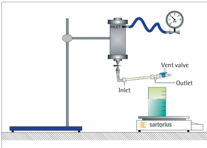
Fig. 2: Experimental set-up of small-scale filtration using Virosart® Media lab module 5 cm<sup>2</sup>
