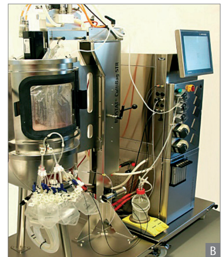
Figure 1: Experimental setup of the cultivation process in the BIOSTAT STR ® 50L. A) Schematic overview of the 3-step cultivation process with cell attachment phase (1: BIOSTAT ® CultiBag RM 20L), cell expansion (2: BIOSTAT STR ® 50L) and cell harvest (3: BIOSTAT ® CultiBag RM 20L). The BIOSTAT STR ® 50L was equipped with two segment blade impellers (SBI) and a ring sparger. B) Experimental setup at the Zurich University of Applied Sciences (ZHAW).
