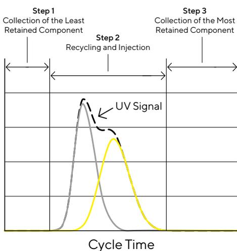
**Figure 3:** Typical Chromatogram for Cyclojet at Steady State.
