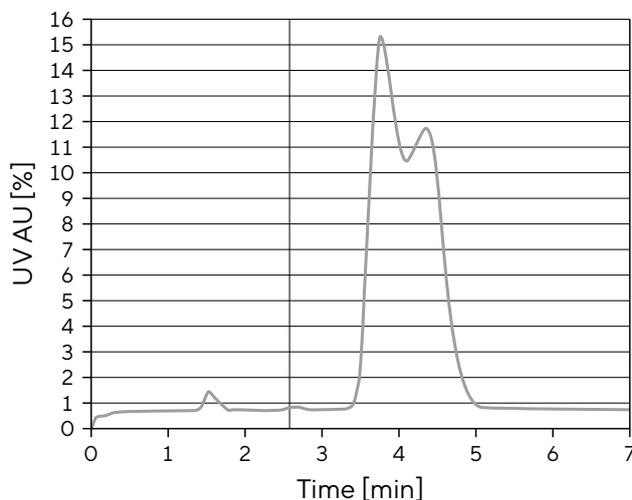
**Figure 5: Overloaded Injections on Preparative Column**
