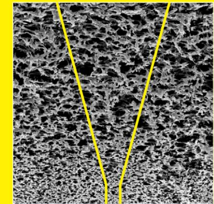
Hydrophilic PES membranes have a high internal porosity. They perform well at high flux with an excellent throughput of aqueous solutions over the entire pH range of 1-14. Their low level of extractables makes them suitable for environmental analysis. Thanks to their low non-specific protein binding, the PES membranes are recommended for filtering biological and pharmaceutical solutions.
