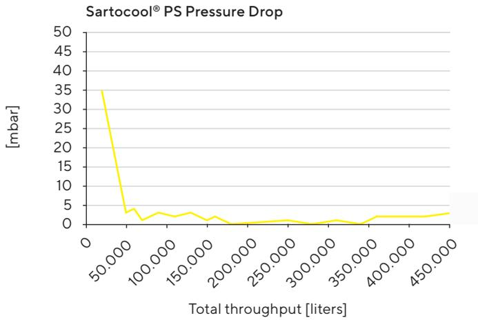
Graph 2: The pressure drop, resulting from the regularly performed integrity tests, were stable over several weeks until the membrane filter cartridges were replaced. Until the end of the  $\beta$ -side test, no increase of the pressure drop was detected. This is the indicator for a robust membrane filter cartridge, which is used in a long-term application. Pressure shocks and regeneration cycles have no negative influence on the product performance.
