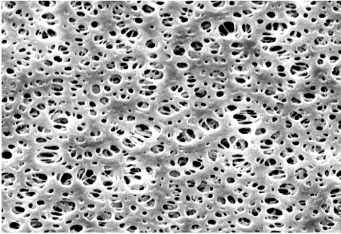
Picture 1: Structure Sartocool® PS Membrane.
