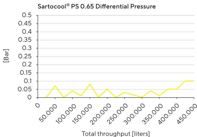
Graph 1: To increase the total throughput, regeneration cycles were performed with caustic soda. After every cycle, the differential pressure reverted back close to zero bar. The membrane was regenerated and the build-up blockage compounds were successfully removed. This is an indicator about the positive regeneration effect. The total throughput for the filter cartridges has been enhanced accordingly.
