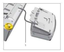
▶ Pull the connection cable (1) between the control unit and the weighing module out of the control unit's retainer and unroll it.
