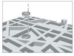
▶ NOTICE Damage to the device from cross-threading! Ensure that the hook for below-balance weighing (1) is inserted straight into the thread.
