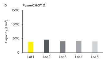
**Figure 3:** Lot-To-Lot Filter Performance Consistency [L/m<sup>2</sup>] Tested With 4 to 5 Different Membrane Lots of Virosart<sup>®</sup> Media Filter for 5 Different Cell Culture Media After 4 Hours of Filtration at 2.0 bar | 30 psi.
