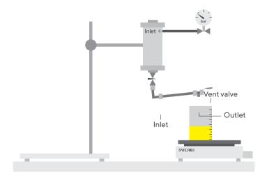
Figure 1: Experimental Set-up of Small-Scale Filtration Using Virosart<sup>®</sup> Media Lab Modules
