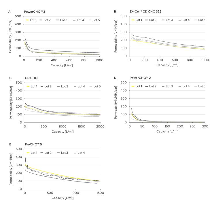
Figure 2: Permeability Versus Capacity. Consistent Lot-To-Lot Filterability Performance for 5 Different Cell Culture Media Tested With 4 – 5 Different Membrane Lots of Virosart<sup>®</sup> Media Filter Each at 2.0 bar | 30 psi.
