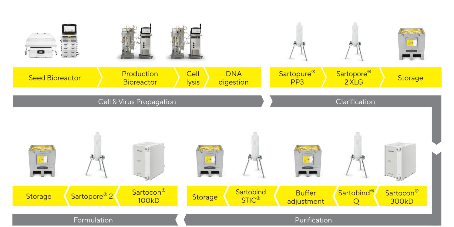
Figure 1: Single-use platform process for adenovirus production
